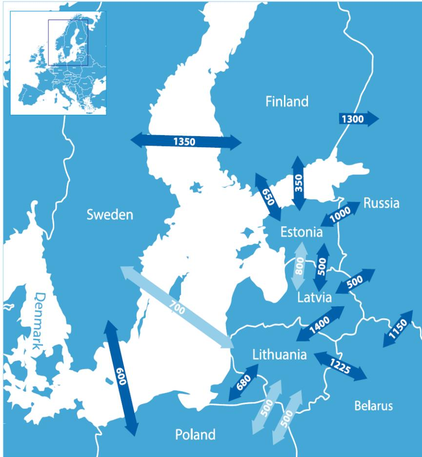
Legend: – projected links (MW), – existing links (MW)
